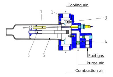
The **burner** is comprised of a two-part burner head, burner tube, gas lance, and electrode.
