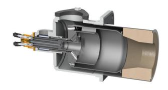
From size B202 H4 upwards each unit may be optionally equipped with a pilot burner. The choice is between an ionization-monitored pilot burner plus additional ionization monitoring of the main flame or, alternatively, a UV-monitored pilot burner. In the latter configuration the main burner flame is sensed through the de-activated UV pilot burner.
