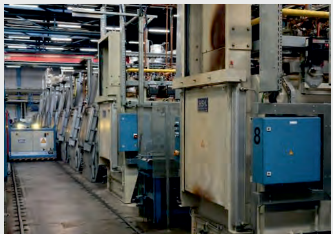
Image 1: Modern hardening shop with numerous chamber furnace plants (modern plants in the foreground)
