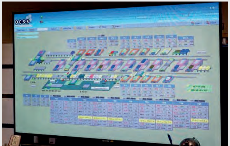
Image 3: Modern control station with a visualization of the entire hardening shop
